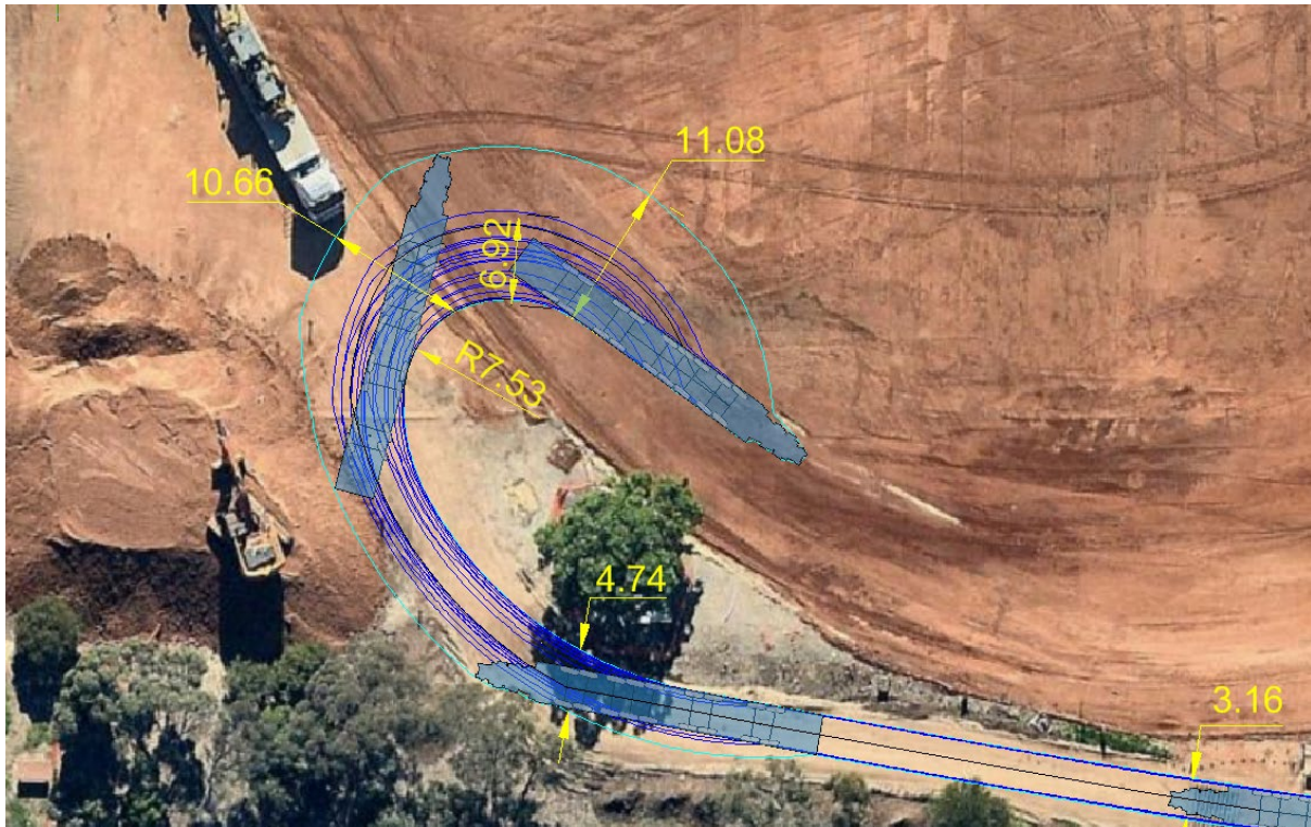
Example 6 – Nine-axle rubber-tired crane swept path analysis
