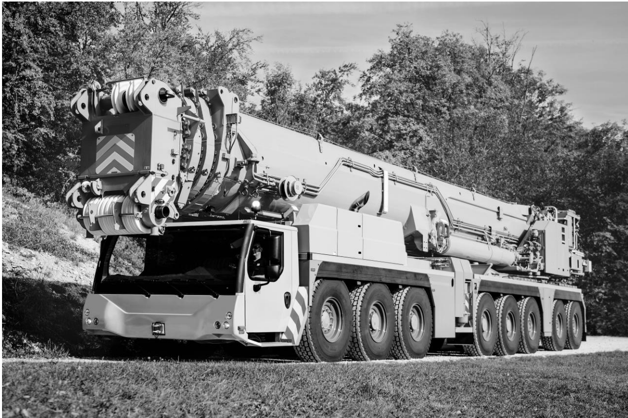
Example 1 – Eight-axle rubber-tired crane
