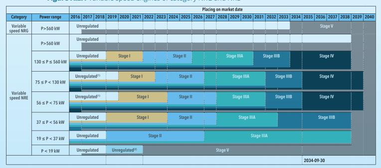
Figure A.2.1 Variable speed engines of category NRG and NRE
