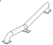
• Bollards / Vehicles Restraints to prevent damage due to impact by other general traffic
