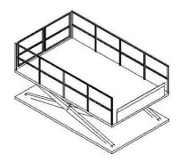
• Handrails if width of bridging method does not fully cover the opening.
