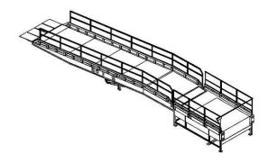
3.2 Height variation, and horizontal gap between loading dock and vehicle deck. Risk of falling between the two whilst moving product/people to/from vehicle.
