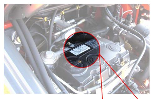
The compliance of engines, installed in industrial trucks on the market, shall be indicated by an information plate, which is visible and durable when fitted on the engine.
