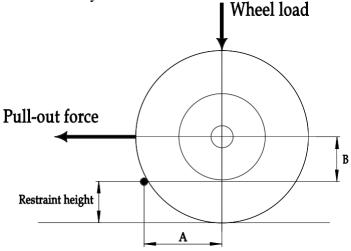
The wheel will drive over the vehicle restraining device when:
