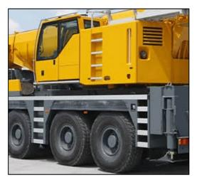
Cabins with a floor higher than 2,5 m (to be measured from ground level) shall be provided with a platform and railings. This platform shall have enough space for at least two persons. Other control stations above 2,5 m height shall be provided with a platform with handholds and railings.
