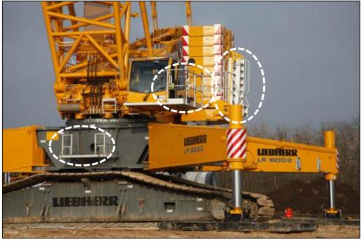
Acc. to the applicable product standard EN13000, the requirements related to the access to the crane cabin are following:
