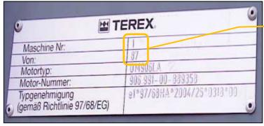
Engine number 1 out of a total of 87 engines permitted under the flexibility-scheme (figures are examples and depend on the particular case
