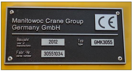
Example of a compliant Machine Plate acc. to 74/114/EC
