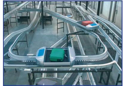
Coordinated by logic controllers and computers running logistics automation software, **automated storage systems in warehouses** enable optimised management of the storage capacity and an efficient use of vertical space.
