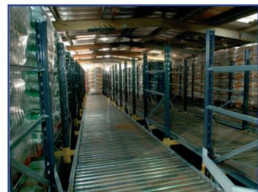
**Mobile pallet racking** (right) is a variation of adjustable pallet racking where the racking is built onto electronically powered bases. It allows the racking to be moved side to side, meaning only one aisle is needed in an area.
