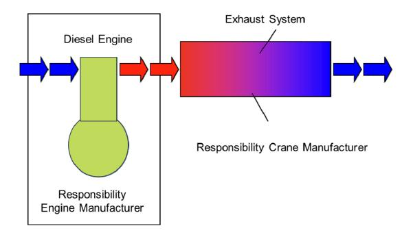
Scope of engine manufacturer's certification for 97/68/EC Stage IIIb
