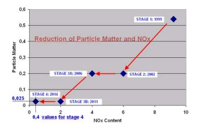
As indicated the level of particulate matter measured in g/kWh will not change when introducing Stage IV; Stage IIIB diesel engines in accordance with 97/68/EC already fulfil the requirements of Stage IV in relation to particulate matter (mass).
